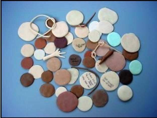
Here is a shot of several samples. Notice the thin strands of clay, some tied in knots. I love this test! Very few brands can pass the knot test. I roll out thin strands of the clay, like a cooked spaghetti noodle. Bake these according to the manufacturer's instructions. Once the clay is cool, bend the strand to see how strong the clay is. If it doesn't snap, then continue and tie the clay into a knot, pulling with a fair amount of pressure.
