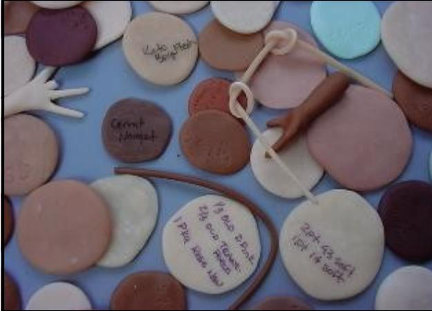
You'll see the clay turn a lighter color where it's strained, but some clays won't break! This is so important so we can create art that will last a lifetime or longer for our collectors. The brands that will pass the knot test are Kato, Puppen Fimo and Cernit.
